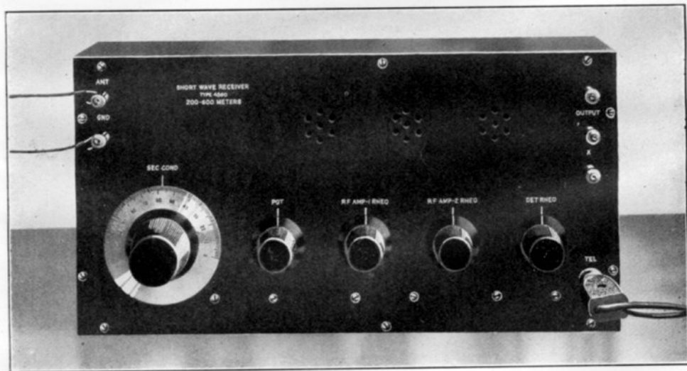
Fig. 1. You will be proud of this receiving set with its two stages of radio frequency amplification and detector. The three binding posts at the right are for connections to an audio frequency amplifier
